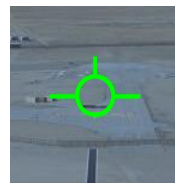
Commanded/Computed Flight Path Vector
