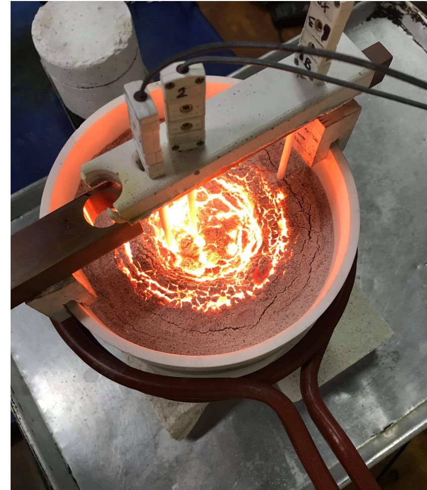
Regolith melt formation by inductive heating (Tests conducted by KSC and RDO Induction, Inc.)
