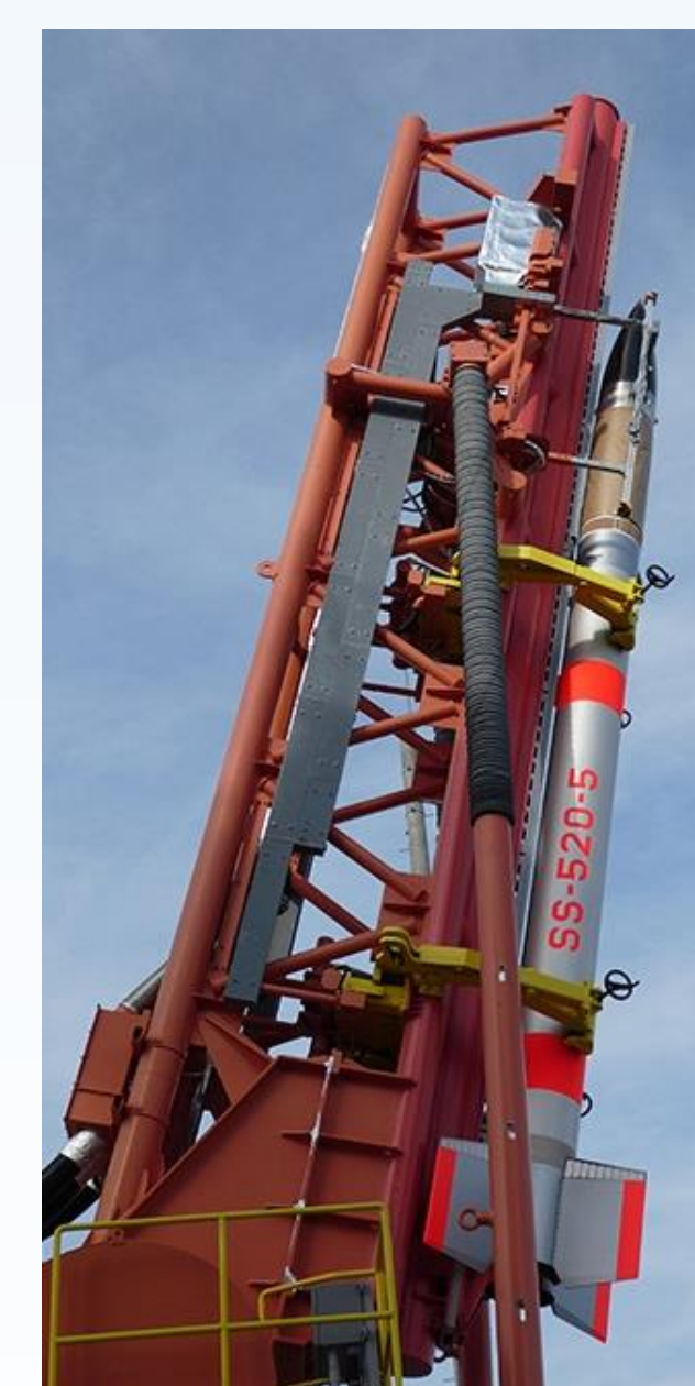
SS-520 orbital booster, at 2.6 tons, the smallest vehicle to launch to Earth orbit
