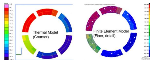
Fig. 12. Temperature Mapping on Structural Model
