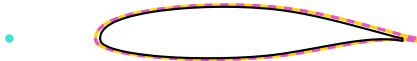
Figure 2: Sketch of the Shen 2 method with one sampling point in front of the airfoil (●). The circulation is computed using the pressure on the airfoil surface (—) and locally redistributed along the airfoil surface (--) when evaluating its influence.
