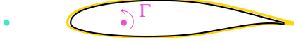
Figure 1: Sketch of the Shen 1 method with one sampling point in front of the airfoil (●). The circulation is computed using the pressure on the airfoil surface (—) and assumed concentrated at the quarter chord (●) when evaluating its influence.
