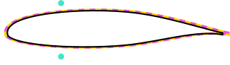
Figure 5: Sketch of the Zhong method with two sampling points adjacent to the airfoil suction and pressure side at the quarter chord location (•). The circulation is computed using the pressure on the airfoil surface (—) and locally redistributed along the airfoil surface (- -) when evaluating its influence.
