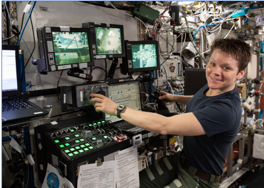
Figure 56. a. Robotic Workstation and Ancillary Controls and Displays; b. Robotic Workstation On Orbit in ISS [ref. 2] (Credit b: NASA)
