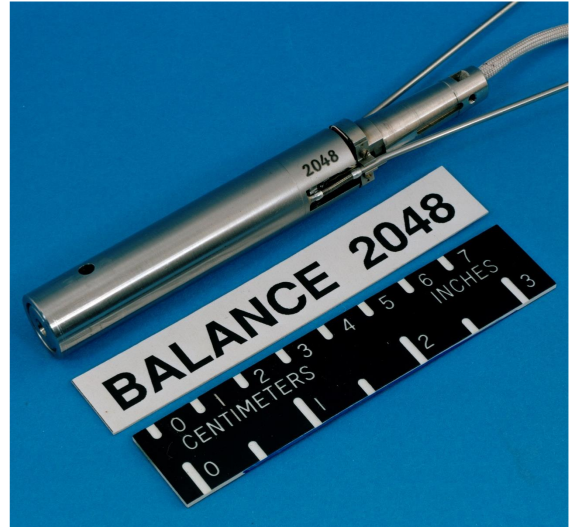
Balance with cooling shield installed.
