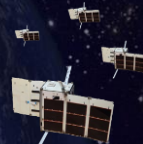
PY4 Four-CubeSat Swarm of PyCubed-Based SpaceCRAFT
