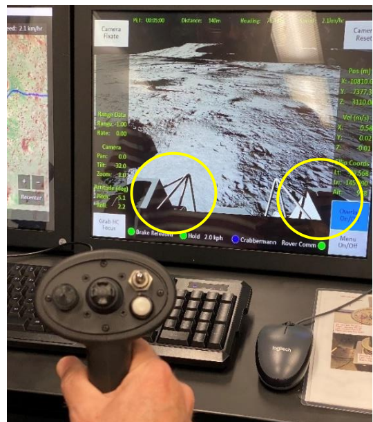
Figure 28. Operators would use the horizontal bars and fenders as guides.
