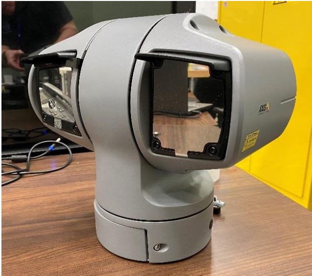
Figure 11. The LTV Mast Camera (Axis Q6215-LE).
