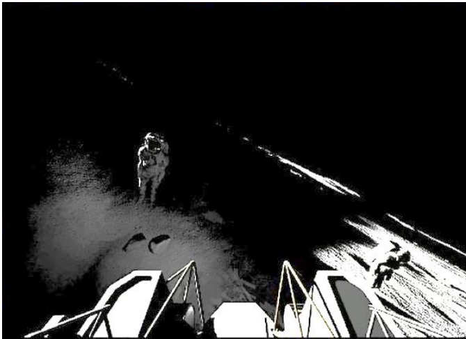
Figure 27. The rover high centered on a crater rim with the crew aiding the remote operator.
