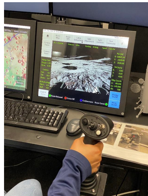
Figure 23. Operators noted the awkward twisting motion of the controller cause wrist flexion fatigue.
