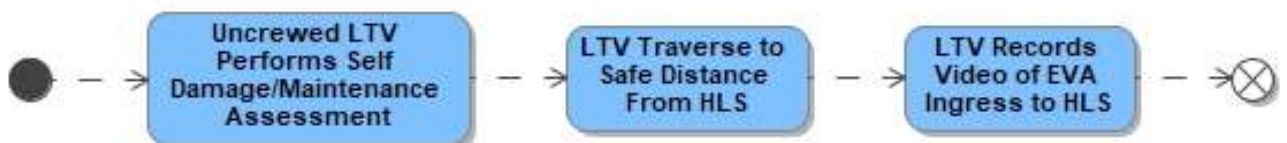
FIGURE 4-26: LTV POST-CREWED OPERATIONS
