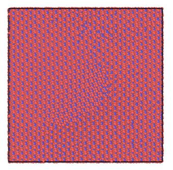
> Crystallization into the rock salt structure was observed.
