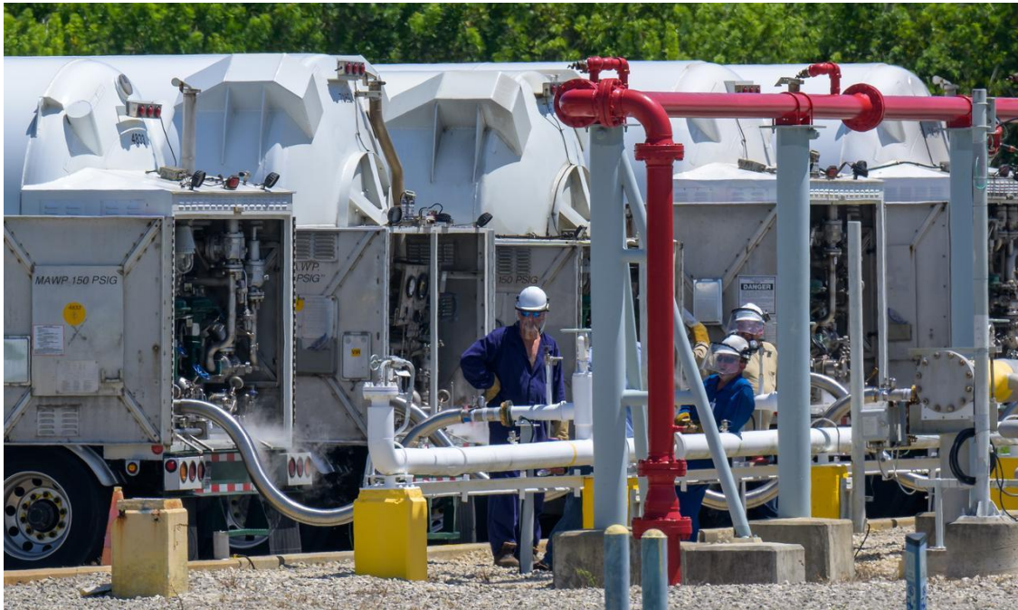
Tanker trucks deliver liquid hydrogen (LH2) for the large sphere at NASA's Kennedy Space Center in Florida, Launch Pad 39B.
