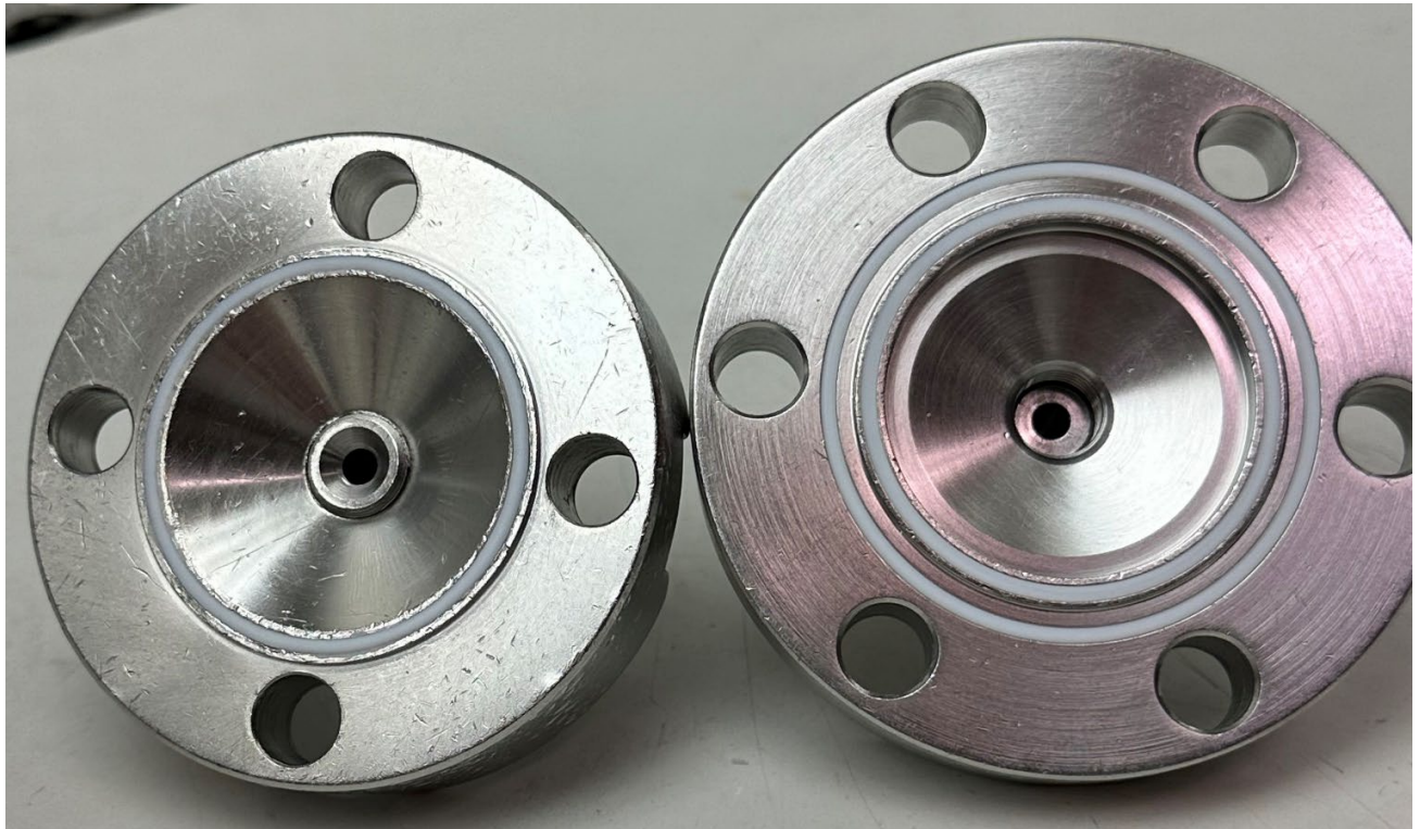
Figure 5. Side-By-Side Comparison of 4-Bolt and 6-Bolt Assemblies
