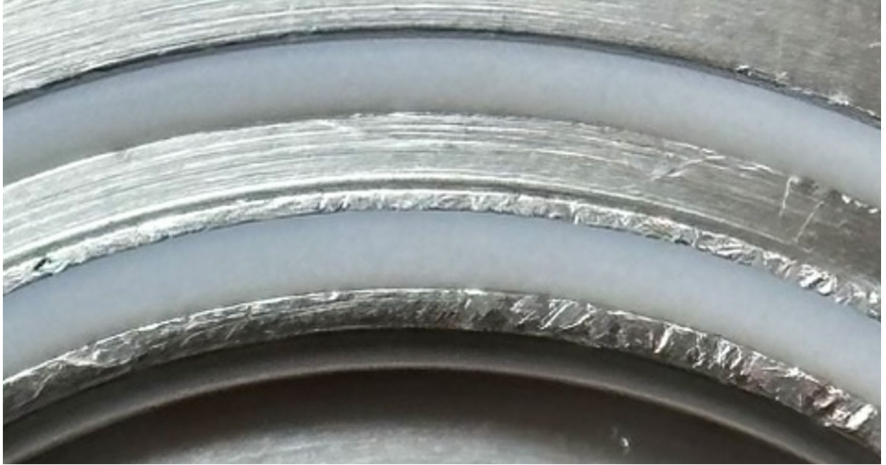
Figure 4. Close-Up of 6-Bolt Assembly Note visible surface wear and abraded metal.
