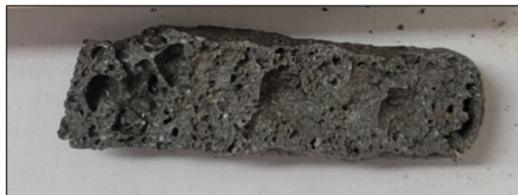
Figure 25. Vacuum sintered sample of CSM-LHT-1G displaying voids created by trapped gas during process.
