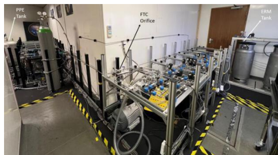
Fig. 4 Gateway Integrated Breadboard Test Rig
