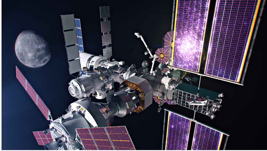
Fig. 2: Rendering of Gateway with Orion docked to the ESPRIT Refueling Module
