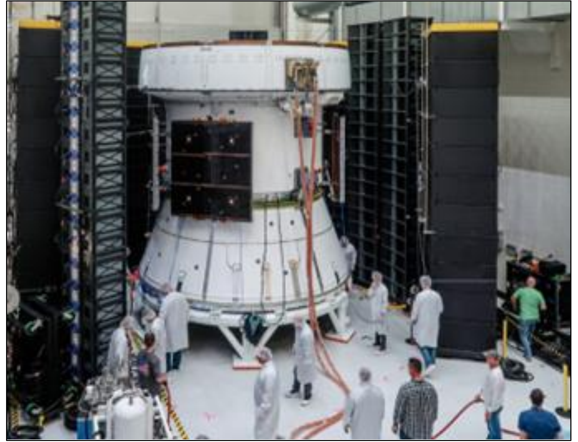
European Service Module for the Orion spacecraft, provided by the European Space Agency.
