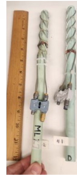
Curved surface print applications: Antennas, strain gauges, sensors
