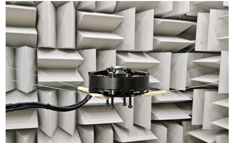
Electric motor noise test in ATL
