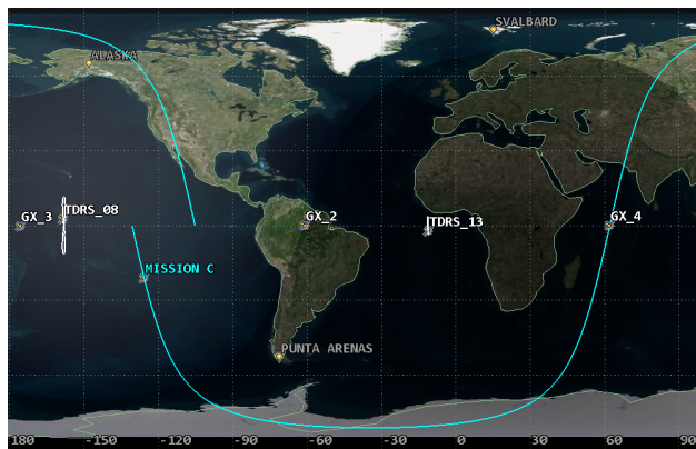
Fig. 16 Ground track of Mission C (blue) compared to planned ground stations (gray) and candidate relay satellites (white).
