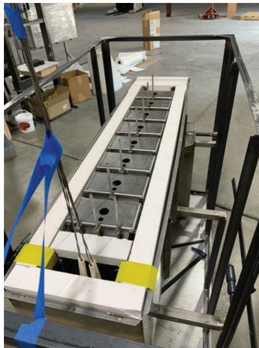
Figure 7.12-3. M-COG Prototype Chassis 2 Configured with Eight Cell Stacks in Series
