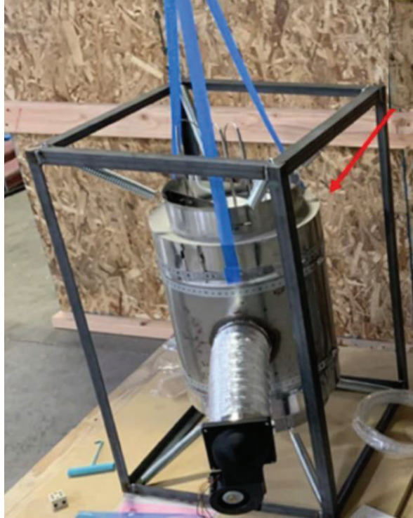
Figure 7.10-1. M-COG with Spring Mounts for Transportation
