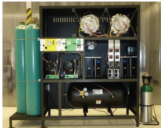
Figure 7.16-1. Forward Operating Base in Afghanistan (left) and Early M-COG System with Mechanical Compressors for Cylinder Filling Operations (right) Note: The M-COG system is shown prior to installation outside the shelters.
