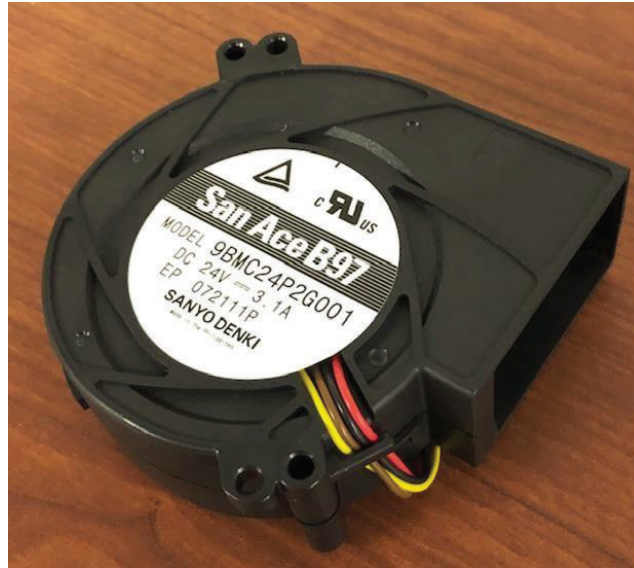
Figure 6.5-2. Blower used in CFC M-COG
