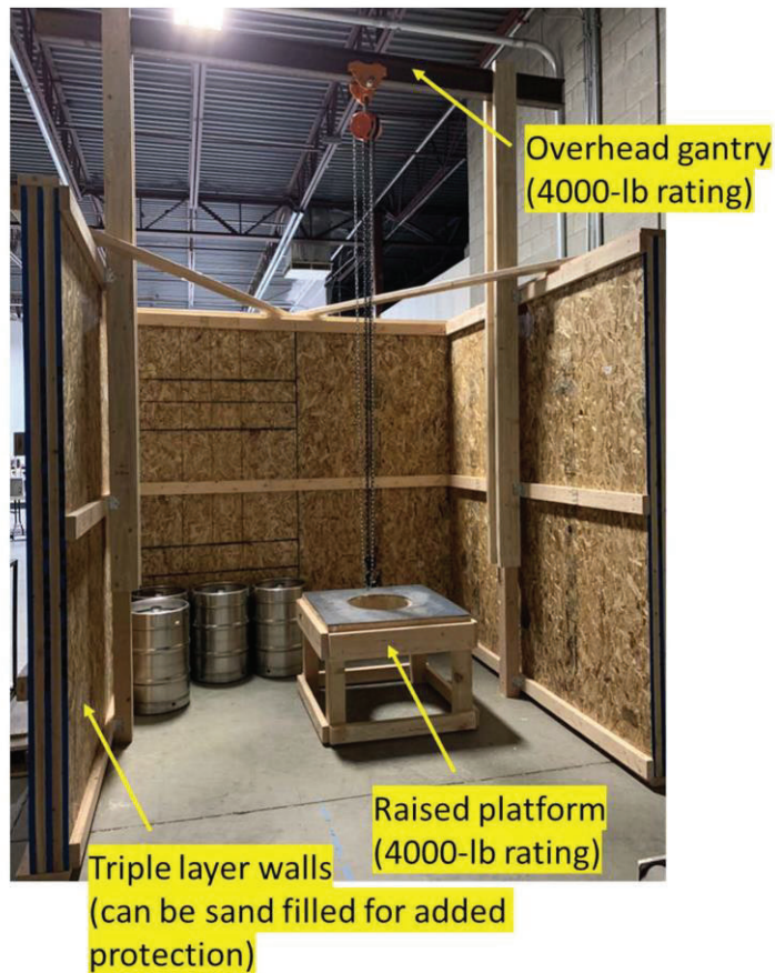
Figure 2.2: Walk-in test bay with raised platform and overhead gantry, and forklift access.
