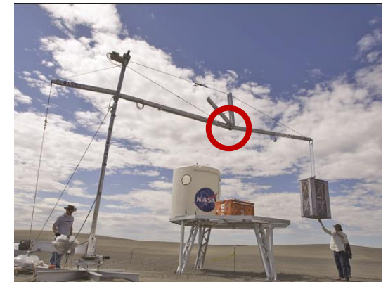
Simplified pin-joint mechanism inspired by Lunar Surface Manipulation System (LSMS)
