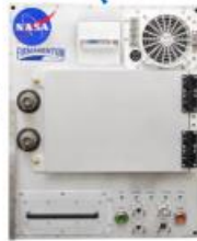
Refabricator – combined plastic materials recycler and printer – for Technology Demonstration on ISS. Image courtesy of Tethers Unlimited, Inc.
