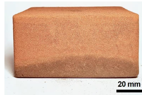
Finished Microwave Brick. Korea Institute of Civil Engineering and Building Technology
