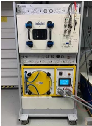
Techshot Fabrication Laboratory ground-based prototype for bound metal deposition. Image from Techshot, Inc. (Redwire)
