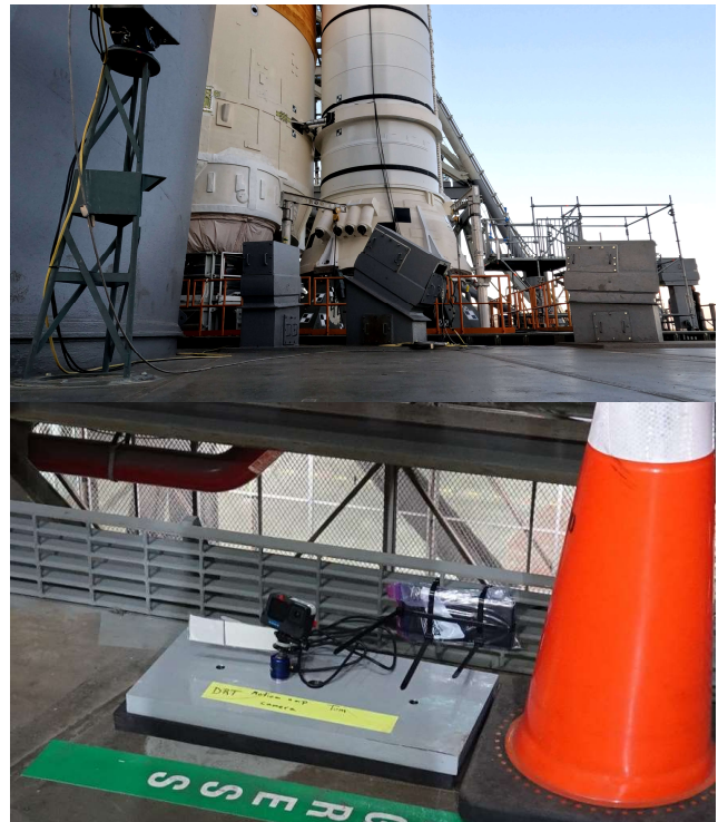
Figure 7. Experimental setup with a GoPro camera during SLS DRRT on the bottom with a screenshot from the GoPro video on the top.
