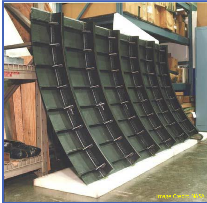
6 ft x 10 ft PETI-5/IM7 Skin Stringer Panel from High-Speed Research (HSR) Program
