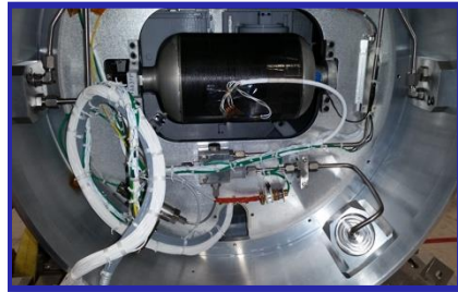
CNT Composite Overwrapped Pressure Vessel Cold Gas Thruster
