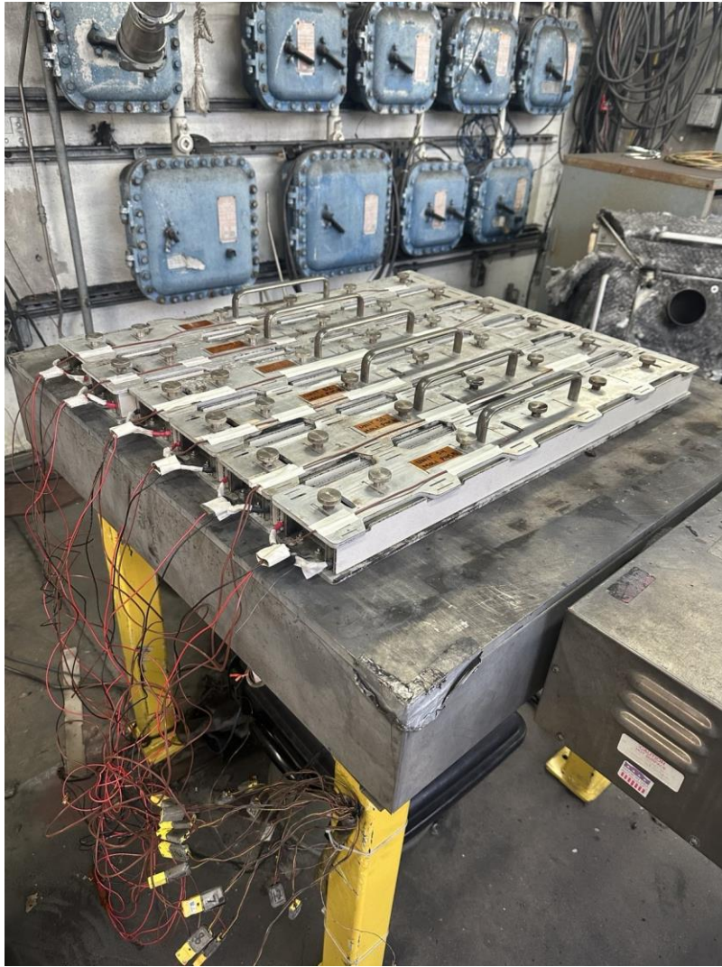
Figure: A 36" X 36" hot plate is used to heat 6 test articles at a time to trigger 60 cells into thermal runaway.
