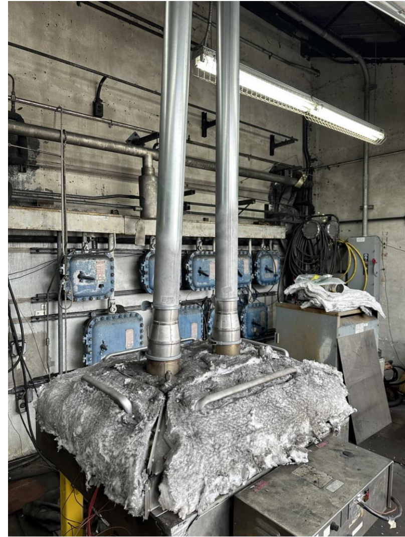
Figure: A 36" X 36" hot plate is used to heat 6 test articles at a time to trigger 60 cells into thermal runaway.
