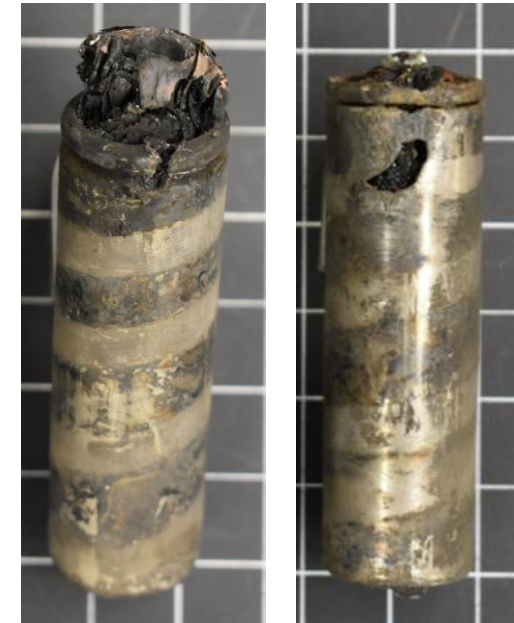
Sidewall Rupture (SWR)
