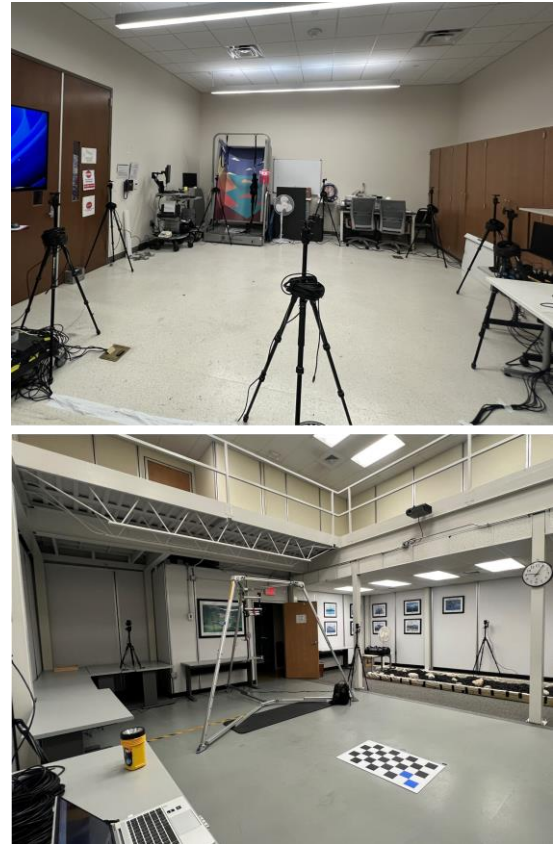
Figure 1. Markerless motion capture volumes. Top: Protocol 1 laboratory setting with eight cameras. Bottom: Protocol 2 field testing with six cameras at the Aerospace Environment Protections Laboratory (KBR, Inc., San Antonio, TX).
