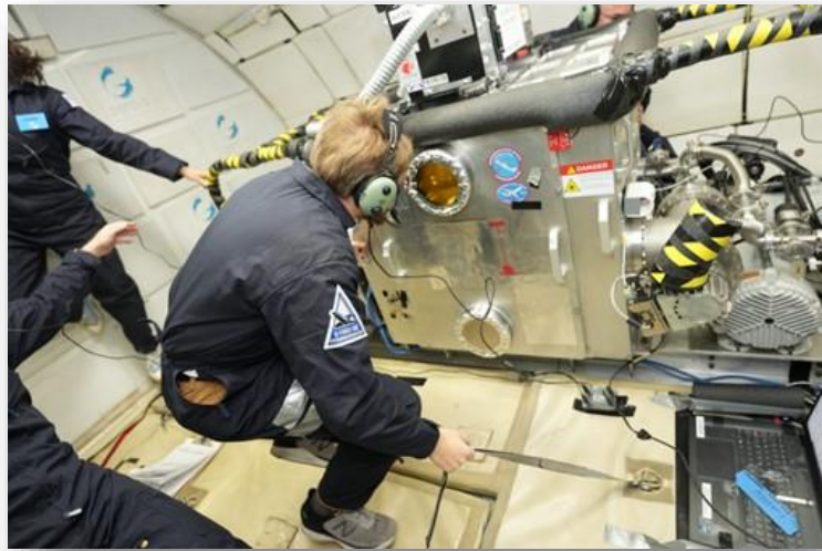
Retrofitted vacuum chamber in flight on Zero-G 727 aircraft
