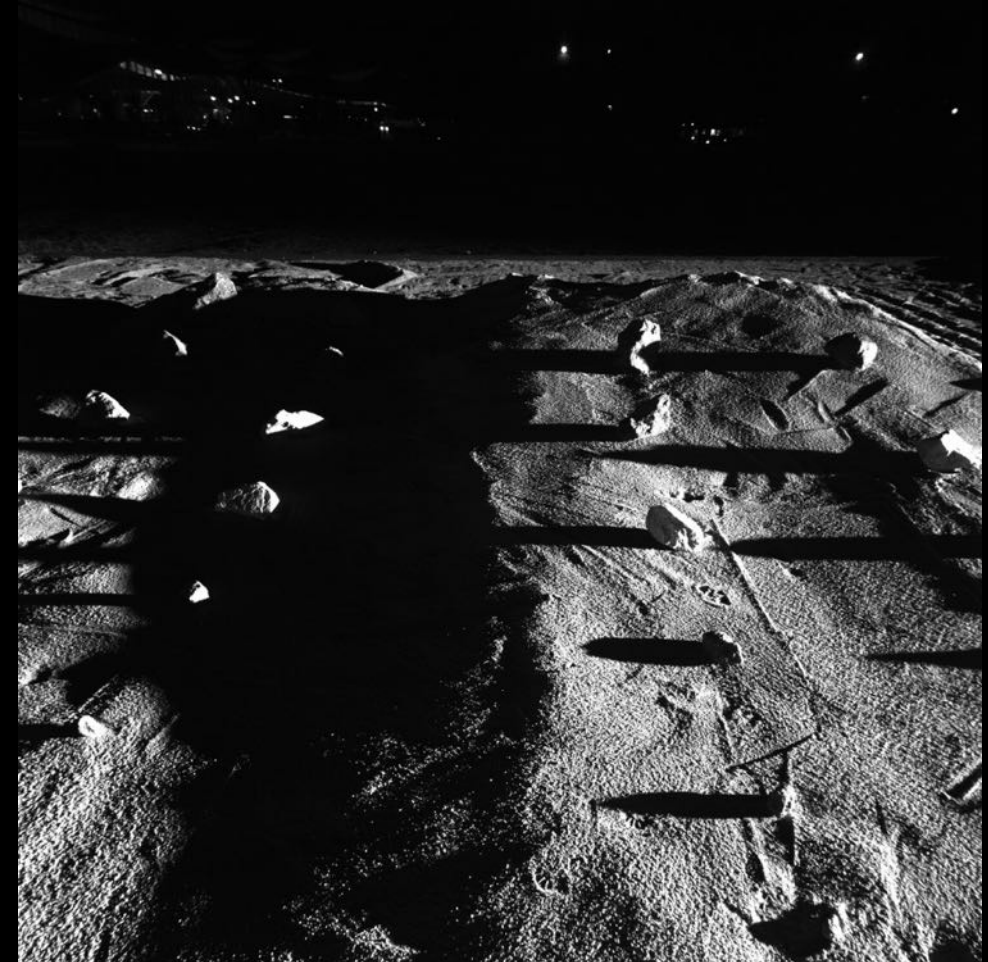
Rock field for hazard map testing with sun simulator on the right
