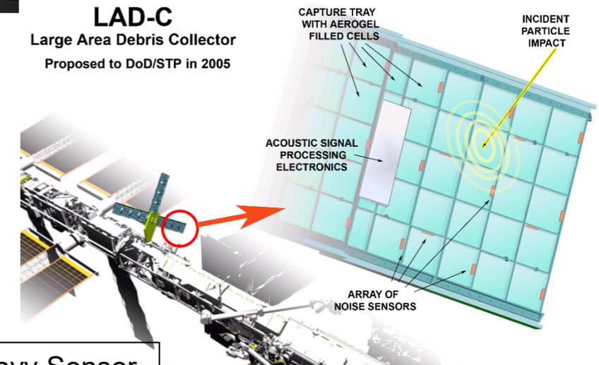
DRAGONS = Debris Resistive/Acoustic Grid Orbital NASA-Navy Sensor
