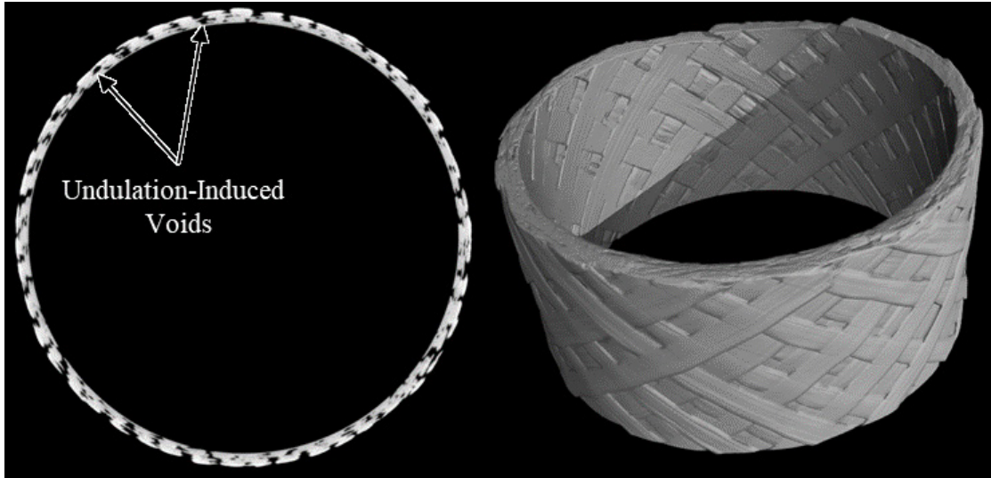
Figure 8.—Computer tomography (CT) scan of tube cross section with notable undulation.
