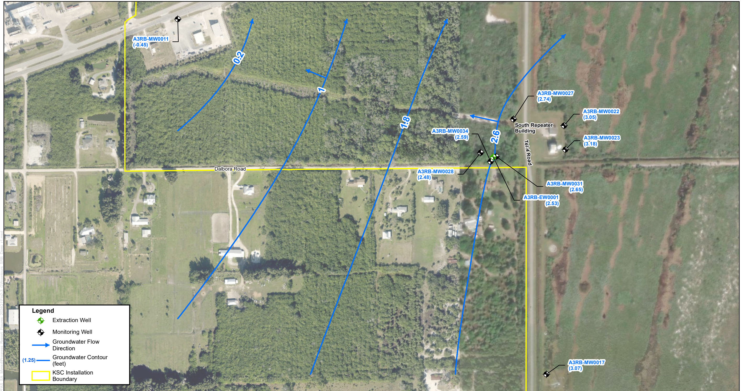
FIGURE 5-3 DEEP GROUNDWATER FLOW DIRECTION FEBRUARY 2024 SOUTH REPEATER BUILDING
