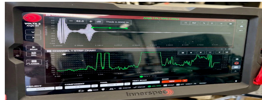
Weld inspection using EMAT system
