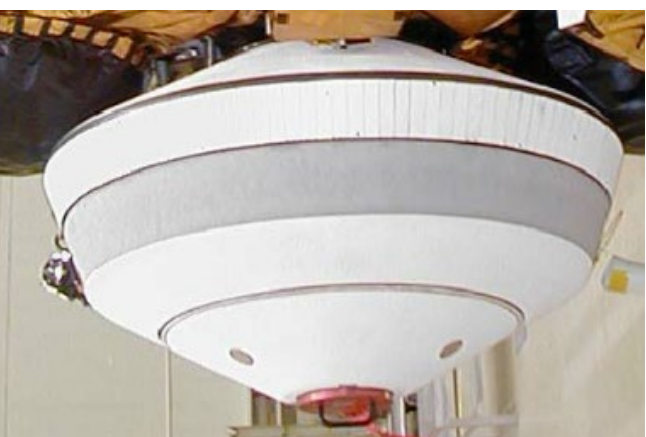
Genesis Capsule with ACC4/Fibeform [NASA]
