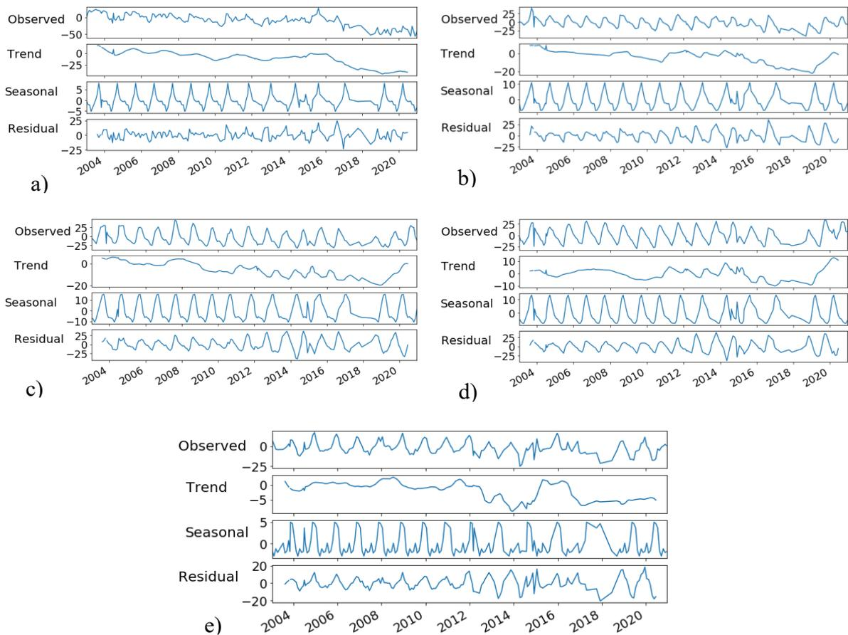
Figure 7. Seasonal decomposition for GRACE grid (a) (30875,73.375) showing decreasing trend in Hotspot I, (b) (26.375,81.375) showing decreasing trend in Hotspot II, (c) (24.125,88.125) showing decreasing trend in Hotspot III, (d) (21.125,82.125) showing no-trend in Hotspot IV, and (e) (8.625,77,125) showing decreasing trend in Hotspot V.
