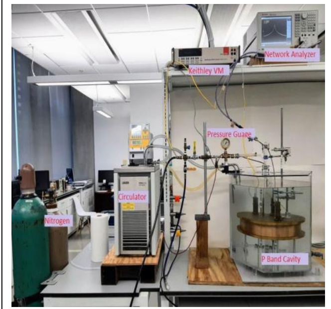
Fig. 1. Experimental setup for the measurement of the dielectric constant of seawater at P-band. The system is the same as used at L- band except for the resonant cavity which is larger and resonant at 0.707 GHz.
