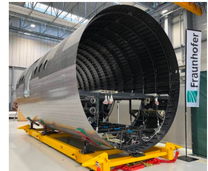
Multifunctional Fuselage Demonstrator, 8m, in situ consolidation, welded assembly, TRL5, 2024
