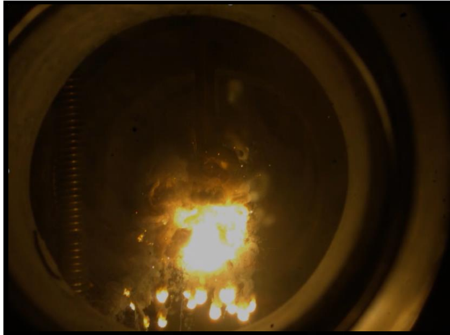
Example of an alloy that burns in pure O 2 , White Sands Test Facility (Courtesy: J. Tylka)
