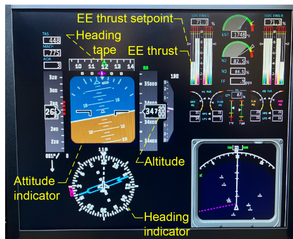
Figure 18.—Annotated pilot display showing relevant aircraft variables. The EE thrust bars in the upper right indicate that EEs 1, 2, 16, and 17 have failed.
