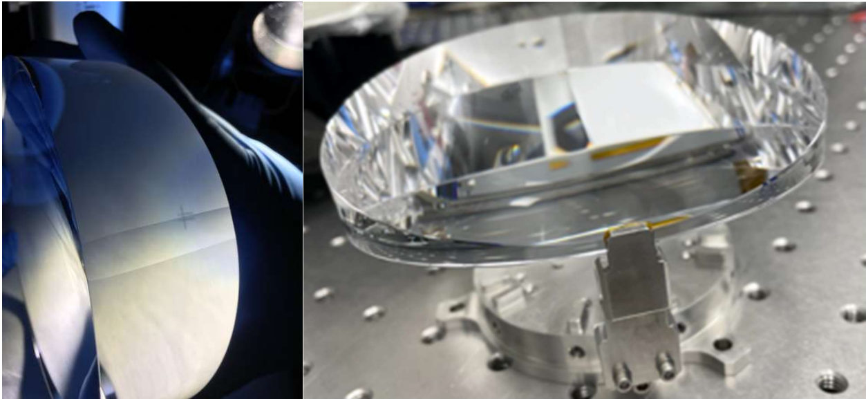
Figure 9. Photos of P2 optical element after completed manufacturing: Two integral flats are polished into the edges of all optical elements. One flat is shown in the center of the left photo. To the right a photo of the entire P2, thin edge in front.
