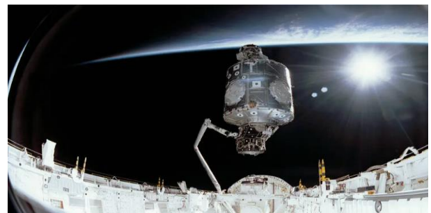
Fig. 2. Berthing of the Unity and Zarya modules started the construction of the ISS in 1998.
