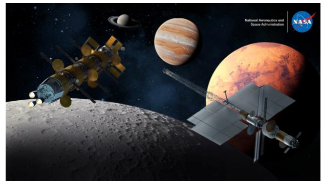
Fig. 1. An artist's rendition of NTP (left) and NEP (right) spacecraft envisioned for deep space exploration.
