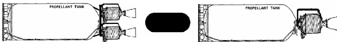
Figure 3.3: Two Engine Configuration with shadow shield cross-section
