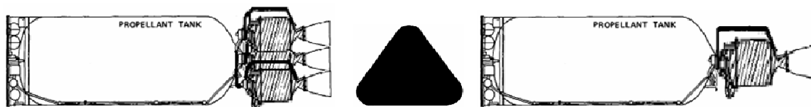
Figure 3.4: Three Engine Configuration with shadow shield cross-section
