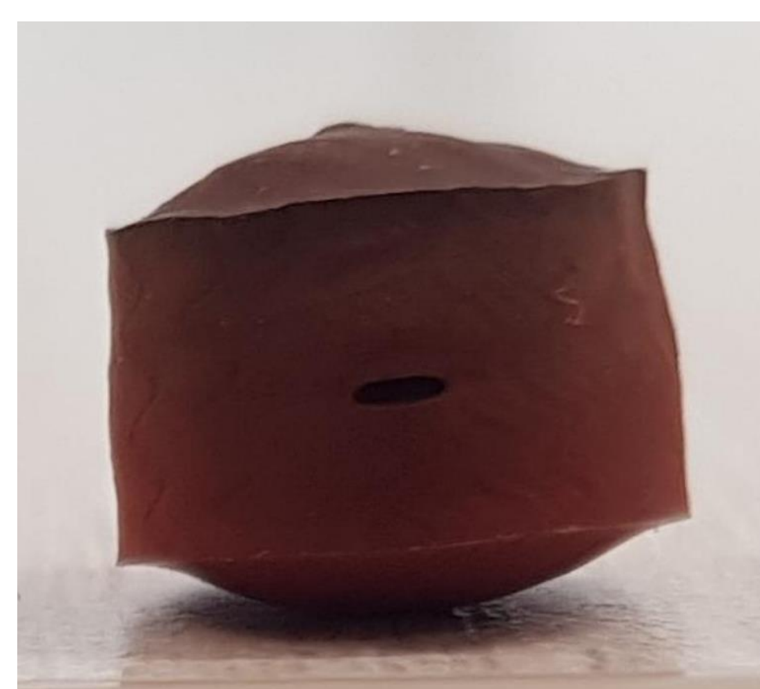
Fig. 3 RTV-560 cylindrical sample heated to ~773K.
