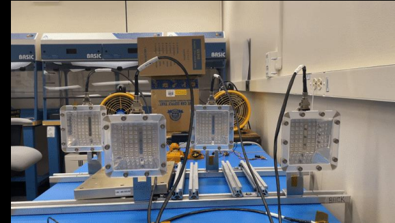
NavLights flashing during burn-in tests
