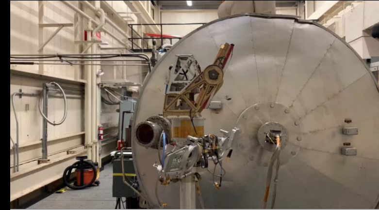
Gimbal Controlled by Flight Mtr Ctrl in TVAC
