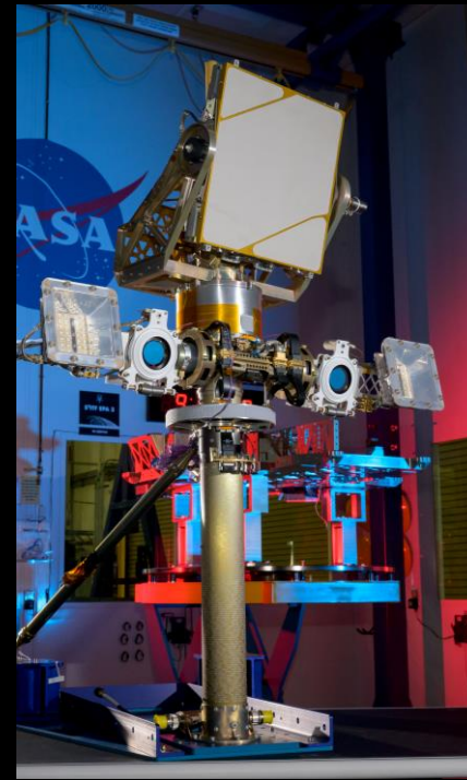
Gimbal Controlled by Flight Mtr Ctrl in TVAC
