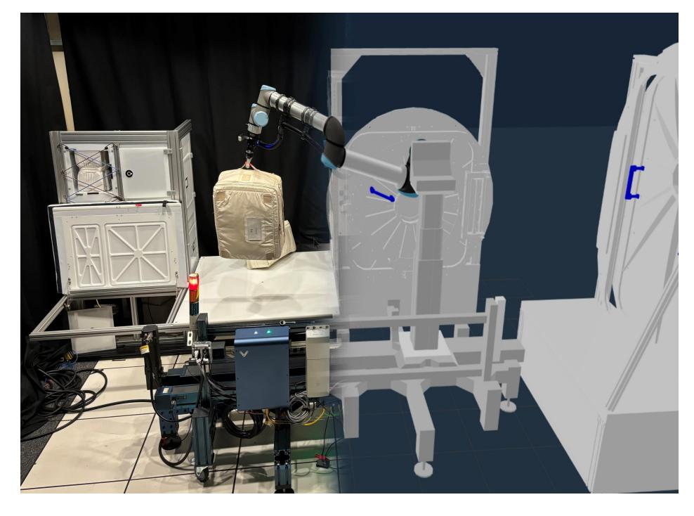
iMETRO serves as a facility for collaborators to test remote operations. Testing with iMETRO remote operations benefits participants by providing scalable test constraints to identify architectural and fundamental design barriers to remote operations with limited bandwidth, high latency, and comm. outages which may not be evident during locally operated lab feasibility demonstrations.
