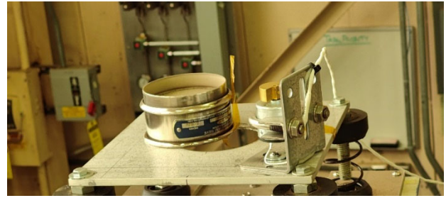
Fig 7. The Overturned Sieve after Test I.
