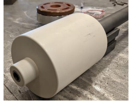
Figure 3: Cold Clamp Adaptor with Embedded Pressure Barrier Tube
