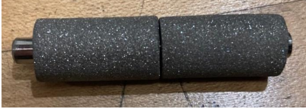
Figure 7: Immersion Rig Inner Insulators
