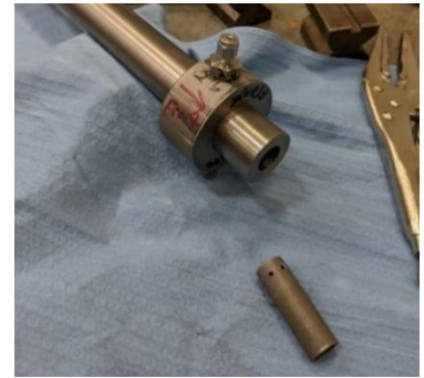
Figure 6: Instrument Ring and Final Tungsten Lattice Segment
