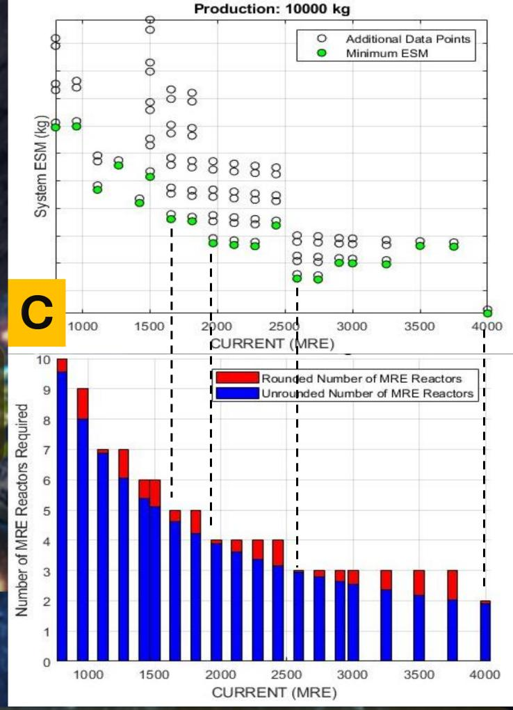
At higher operating currents, the MRE reactor is more efficient and has a higher rate of oxygen production (bottom graph), but a larger inner diameter of the reactor is required to avoid wall melting (top graph).
