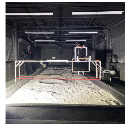
Sliding gantry over LHS-1 terrain
