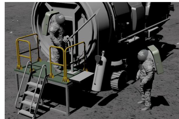
Tank lift via davit
