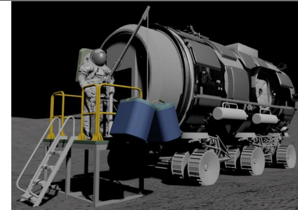
Rendering of CPC transfer by davit 2 at a time
