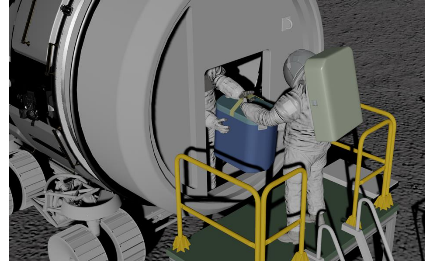
EV1 transferring a CPC across the hatch to EV2
