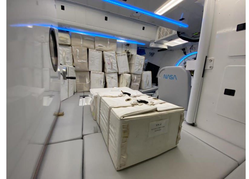
A soft-sided Cargo Transfer Bag (CTB), the traditional container for transferring cargo around inside or between pressurized spacecraft
