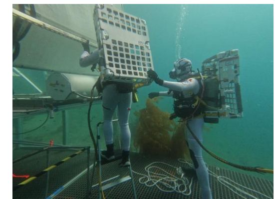
Use of step stool for tank hoist connection/disconnection at vehicle mount.
