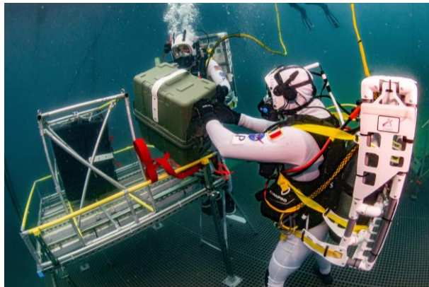
Use of step stool to unload CPCs from 1m LR (required 2 crew members)
