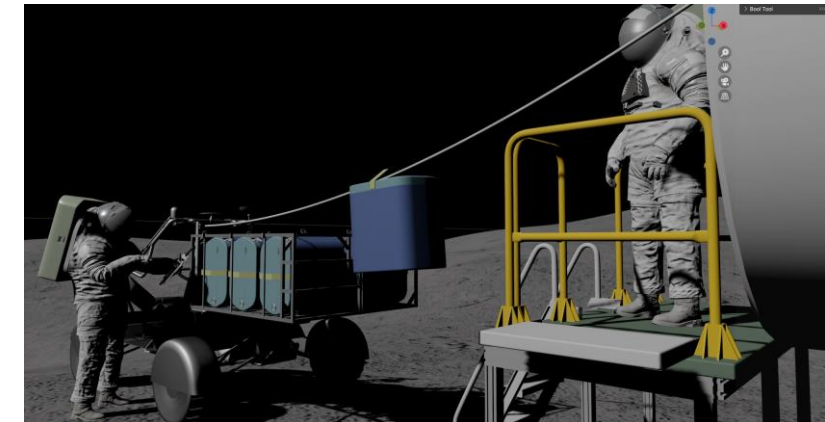
Artist concept of crew utilizing a zipline to transport a CPC to the MPH porch level
