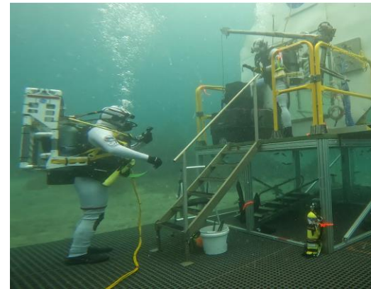
Porch with 4 CPCs and davit in place
