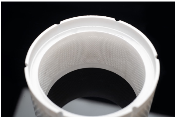
Figure 14: The QUEEN V1 Bulk Absorber Inlet Duct Acoustic Liner
