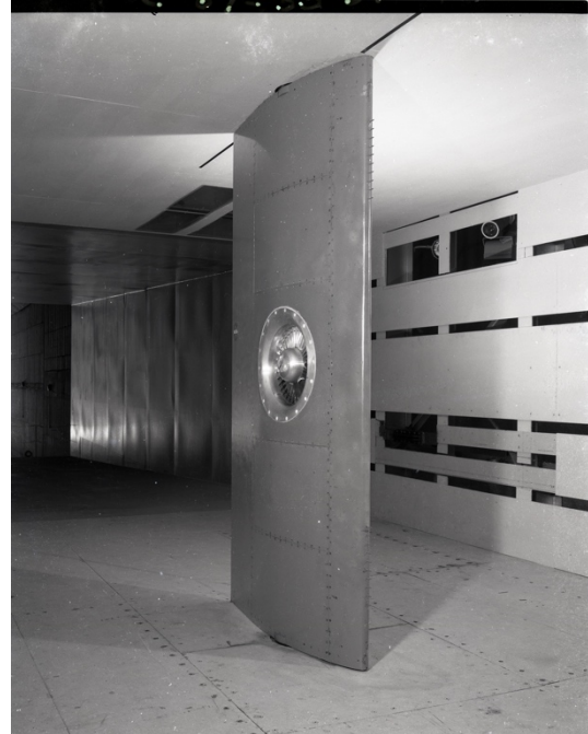
Figure 5: Fan in Wing Model in the NASA Lewis 9- by 15-Ft Low Speed Wind Tunnel; Image: NASA 1969-C-03531, see Reference 11, Figure VI-32, page 167.
