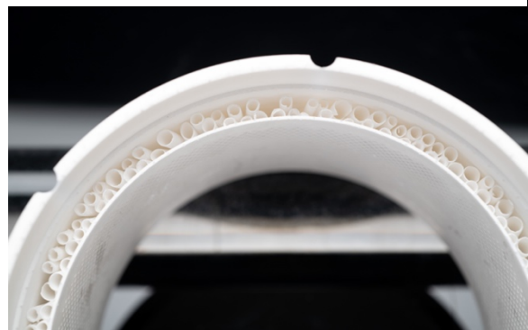
Figure 15: The QUEEN V1 bio-inspired Broadband Acoustic Absorber Inlet Duct Acoustic Liner
