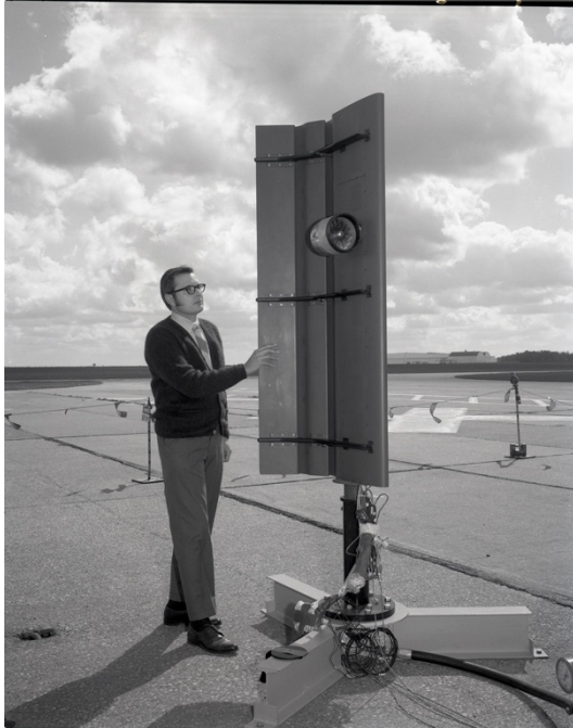
Figure 4: A Blown Flap Model; Image: NASA 1970-C-03034; see Reference 11, Figure VI-32, page 201.
