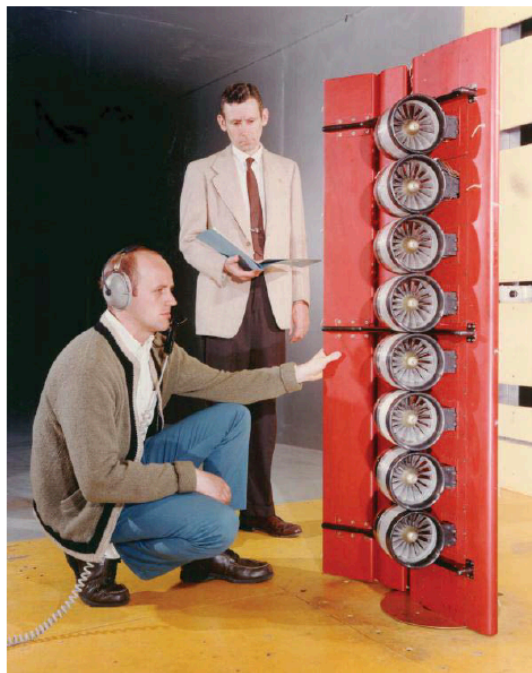
Figure 2: A Blown Flap model in the NASA Lewis 9- by 15-Ft Low Speed Wind Tunnel; Image: NASA 1970-C-01199; see Reference 2.
