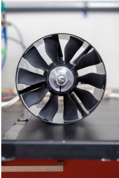
Figure 7: The COTS EDF with rotor and carbon fiber shroud visible, forward looking aft.
